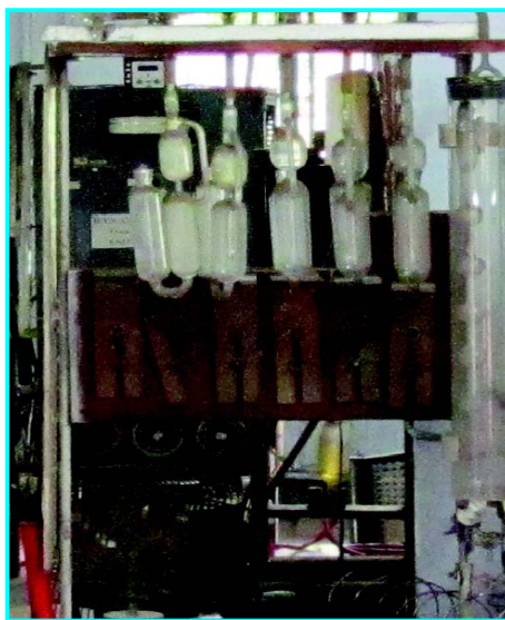
OSRAT Apparatus used for determination of % CO, CO 2 , CH 4 & H in Syn Gas
