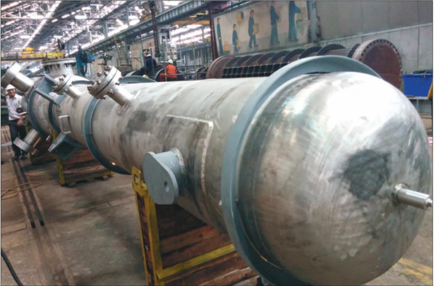
Final checking of full assembled Ammonia Pre heater for RCF Thal.
